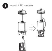
\* For this product, the cable with a plug that comes with the LED module is not needed. Please remove it first and then use the LED module.
